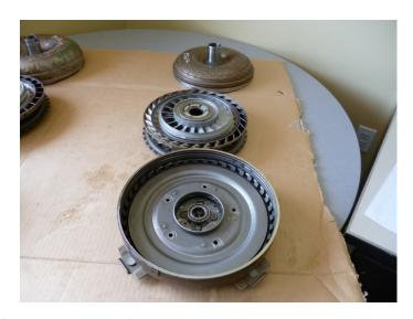
These pictures show you TWO different diameter converters. **No parts** will interchange when building these two different diameter converters.
