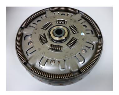
Turbine, Turbine Hub and Damper Assembly – this is a unit.
