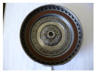
This picture shows the larger cover with the piston removed by drilling out the stands in the cover. This is also **NOT** a good idea.
