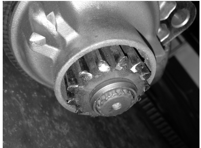
Intermediate Adapter Housing (comes w/o an oring, if installed without it will cause engine oil leak)
