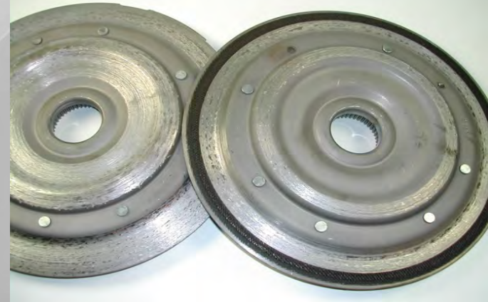
Excess apply psi. = Bent TC piston
