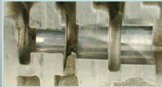
Valve bore wear
