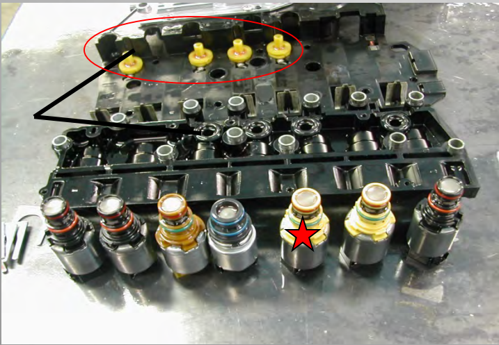
Gen I, Late thimble and o-rings. Star is TCC solenoid
