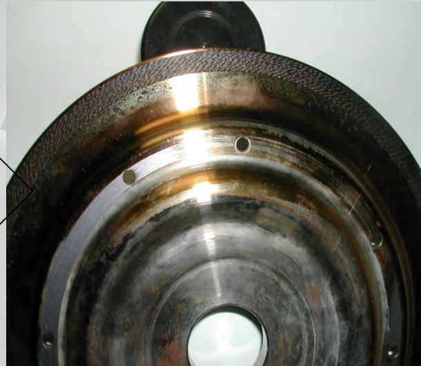
Excess slip or poor pressure control = heat.
