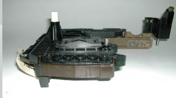
Audi- ZF 6, TCM, Contamination and terminal solder issues.
