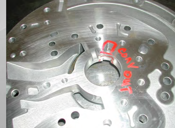
ZF 6- Pump circuit cross leaks.
