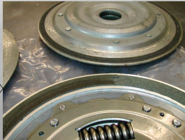
Excess apply pressure = piston distortion & lining failure.
