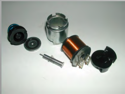
6T30, solenoid contamination
